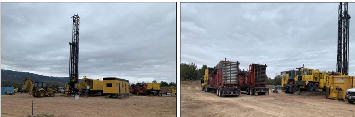
Atlas Copco RD20 Drill Rig and Associated Equipment on location at Amerigo Vespucci #1 well site
