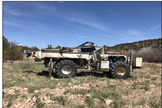
Seismic buggy drill machine
