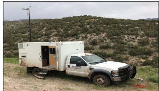
Seismic Recording Truck
