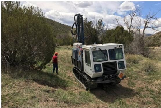
Seismic track drill machine
