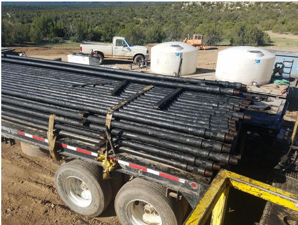
Figure 1: Amerigo Vespucci #1 Well: 154 joints of drill string (4,620 feet) covered in crude oil
