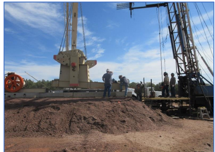
Figure 5: Running pump-rods into the Amerigo Vespucci # 1 well
