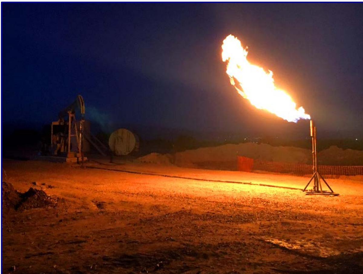
The Magellan # 1 well flaring gas as the well commences oil production
