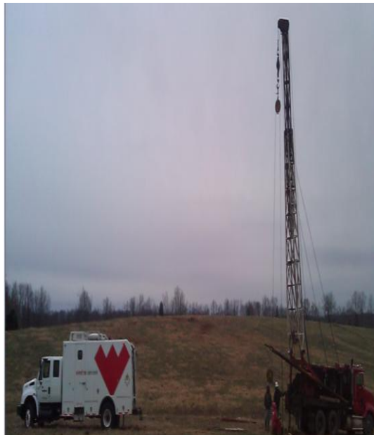
WEATHERFORD WIRE SERVICE LOGGING THE WELLS WITH GAMMA RAY, DENSITY PEROSITY, NEUTRON DENSITY, TEMPERATURE LOG, PE EFFECT & DEEP AND MEDIUM INDUCTION
