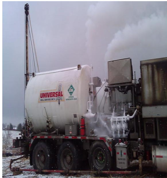
UNIVERSAL WELL SERVICES- NITORGEN TANK TRUCK ON SITE
