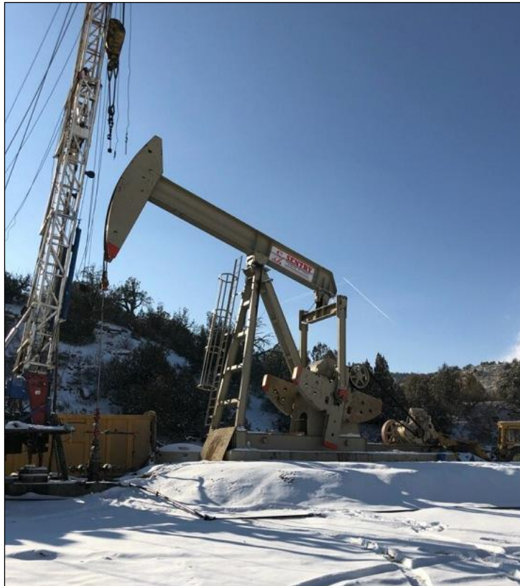
Figure 1: Pump jack installed on the JW #23-25 Well
