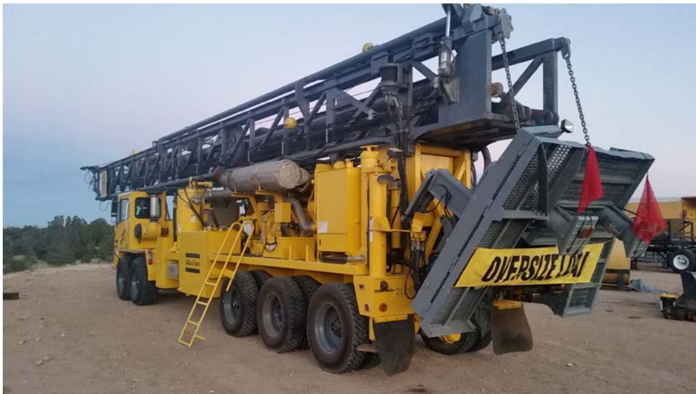
The Atlas Copco RD20 Range 3 drill rig has arrived on location
