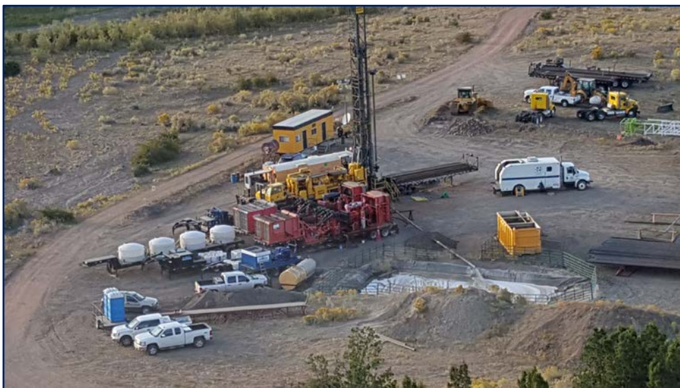
Drilling operations underway on the Columbus #1 well targeting oil production from the Pierre Shale formation
