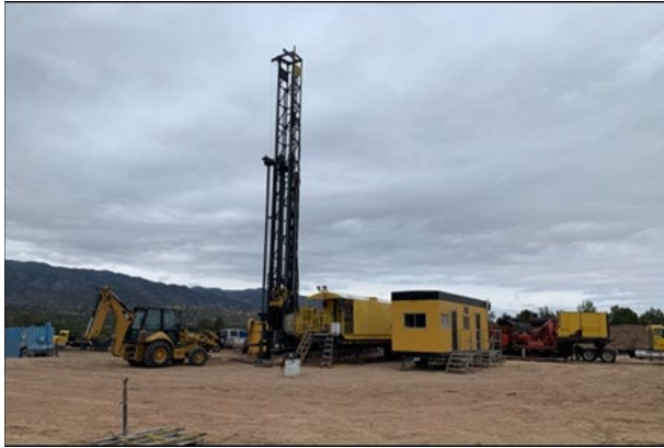
Atlas Copco RD20 Drill Rig and Associated Equipment on location at Amerigo Vespucci #1 well site
