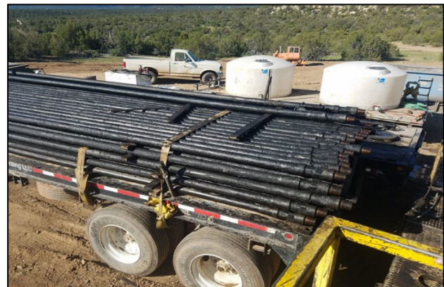
Amerigo Vespucci #1 Well: 154 joints of drill string (4,620 feet) covered in crude oil
