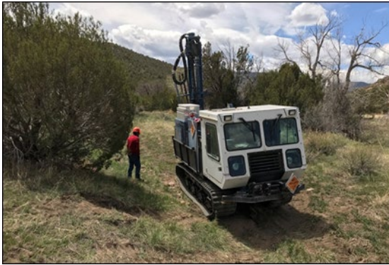
Seismic track drill machine
