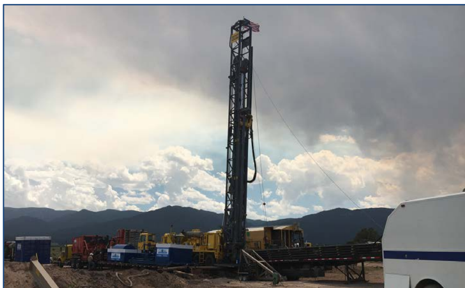
The Math Energy drill rig drilling ahead on the Magellan#1 well
