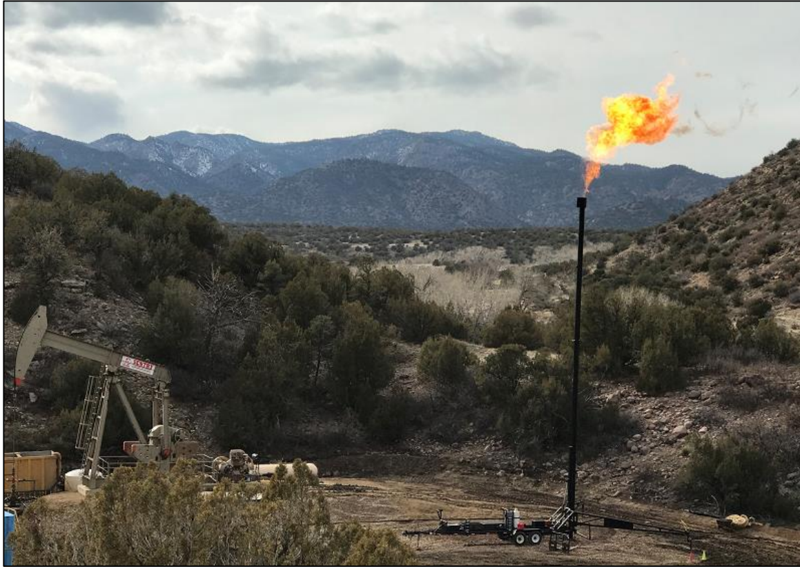
Figure 1: J.W Powell Well: 40-foot Gas Flare During Production Test
