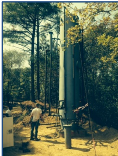
OIL AND GAS HEATER TREATER BEING TESTED
