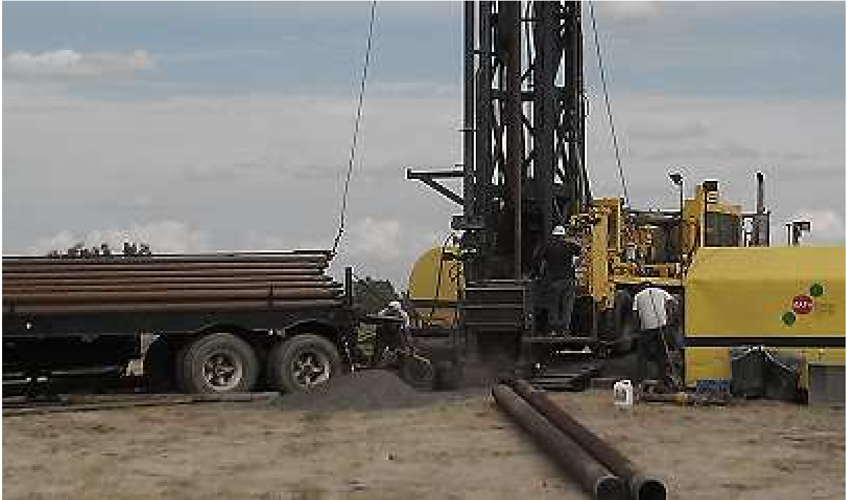
Kentucky 24 Hr drilling operations; Math Energy RD -20 drilling rig drilling Tapp A4 well. The well was drilled to approximately 2900 ft deep and was drilled in a record time of 5 days. Hydrocarbons were intersected and the Company is preparing a low cost frac to maximise production
