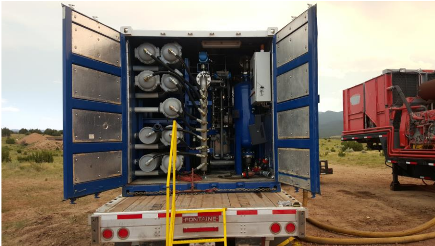
Nitrogen membrane unit generates 94% Nitrogen at 1500psi
